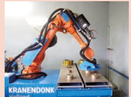
2. Robotic arms pick up flanges from the material rack
