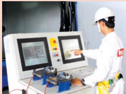
1. During the pipe spool fabrication process, the operator selects the desired spool to fabricate and imports relevant data files to the machine to activate it for the production job
