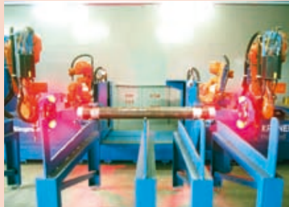
3. The flanges are aligned to the pipe using a vision camera (left) and an 8-point position sensor (right)
