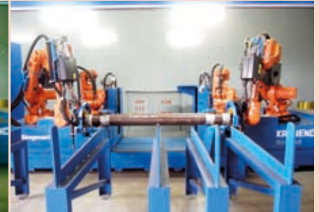
3. The flanges are aligned to the pipe using a vision camera (left) and an 8-point position sensor (right)
